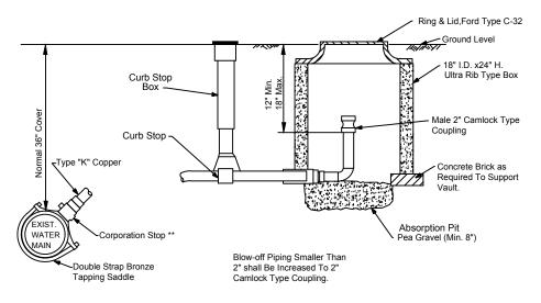
\*\* Taps on mains which utilizes a cathodic protection system shall require an isolation corporation stop
