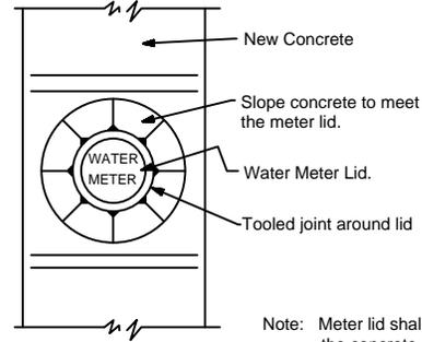
Note: Meter lid shall be flush with the top of the concrete surface. The concrete surface shall be tapered to provide a smooth transition to the meter lid. A tooled joint shall be formed around the meter lid.
